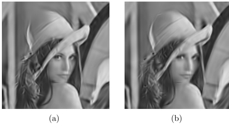
Figure 5.18: Scrambled Matching Pursuit results. Figure (a) is the reconstruction of LENA image with 450 atoms given by the standard flavor of Matching Pursuit and figure (b) is the Scrambled Matching Pursuit reconstruction with the same number of atoms. Results:
