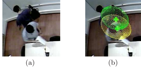
Fig. 2. Particles from the tracker A (yellow ellipsoid) falling into the exclusion zone of tracker B (green ellipsoid) will be penalized by a multiplicative factor \alpha \in [0, 1] .
