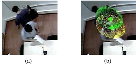
Fig. 3. Particles from the tracker A (yellow ellipsoid) falling into the exclusion zone of tracker B (green ellipsoid) will be penalized by a multiplicative factor \alpha \in [0, 1] .
