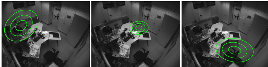
Fig. 11.7. Three Gaussian mixture components obtained from data-driven clustering. They represent areas where users often sit.
